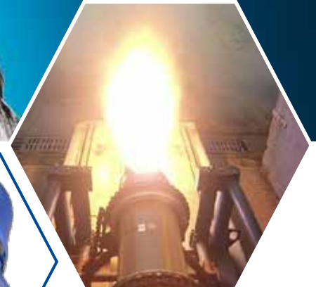
Rocket motor filled with RAM-mixed propellant
